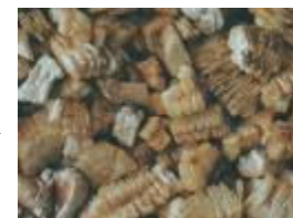
Zonolite - asbestos containing insulation
